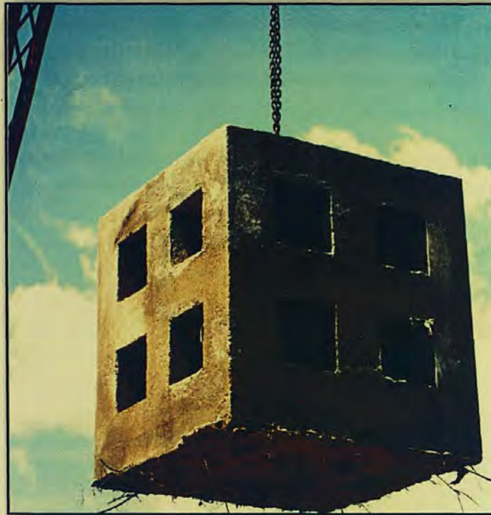
Figure 5 : A side view of a 3.2 tonnes concrete anchor
