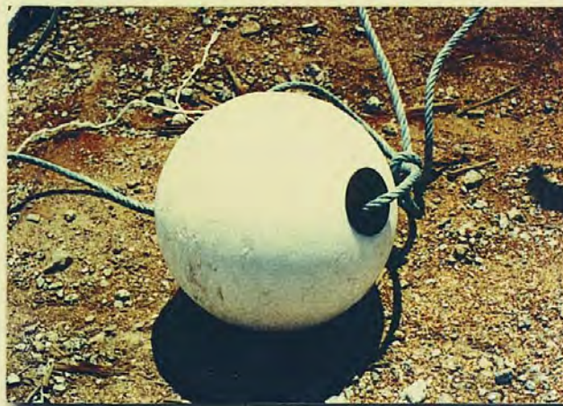
Figure 4 : Styrofoam floats used as surface float. The size of each floats is about 33 cm diameter
