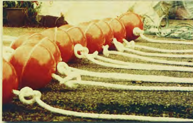
Figure 3 : The submerged floats used for these ARFADs. The size of each float is 30.4 cm diameter with a 2.5 cm hole in the middle
