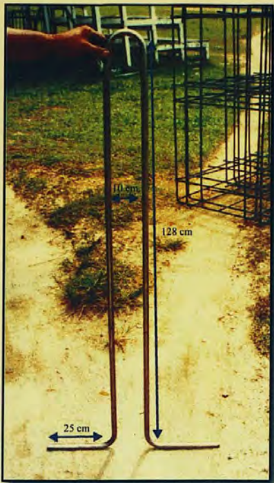
Figure 6 : Details of anchor attachment point (bail). Total length of round stock is approximately 316 cm
