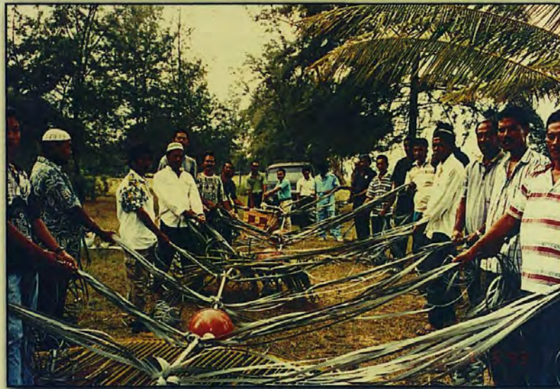
Figure 13 : Plastic strips were knotted at the mid-point of the 6 m length rope so that each of the two ends is 3 m long
