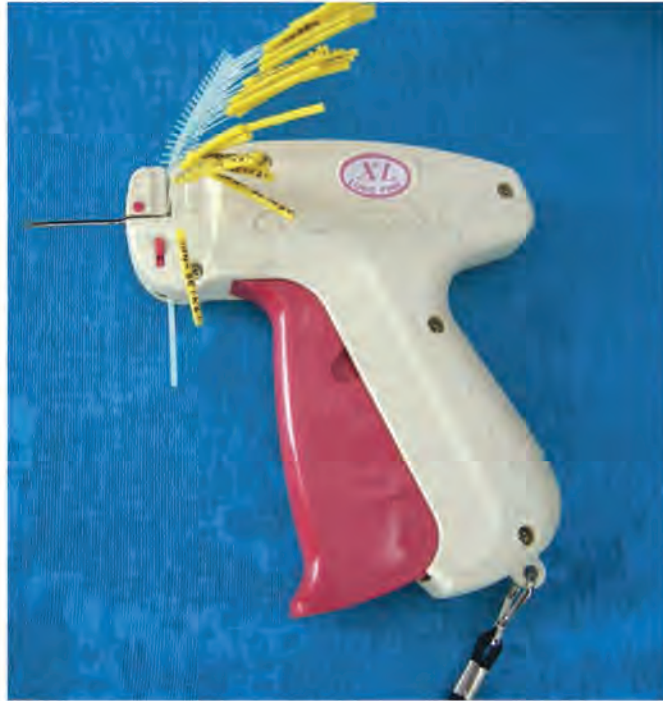
Figure 8: The applicator with T-bar 2 tag ready to be used in fish tagging operation.
