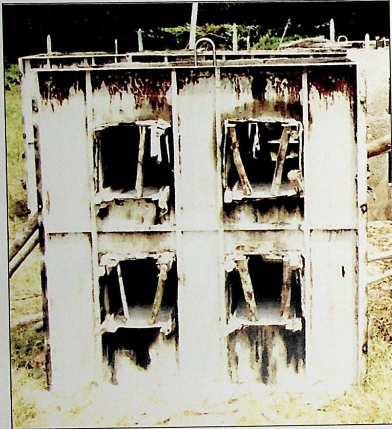
Figure 9 : A side view of the iron mould for concrete anchor
