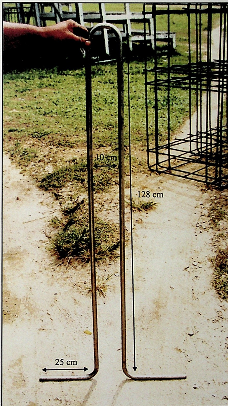
Figure 6 : Details of anchor attachment point (bail). Total length of round stock is approximately 316 cm.
