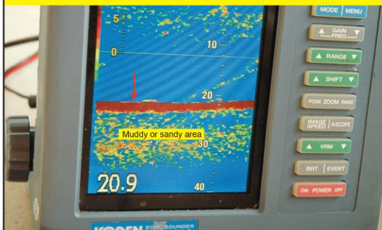
Contour of sea bottom from Echo sounder image
