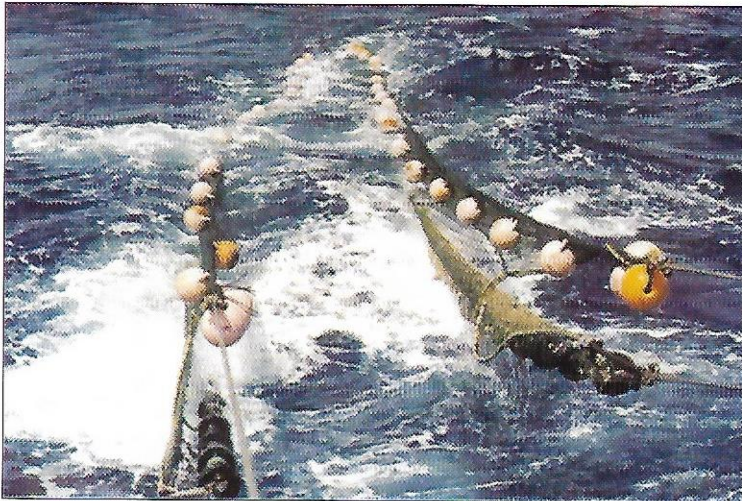
Plate 2: Hauling of the high opening bottom trawl net after one-hour duration at a trawling speed of four knots.
