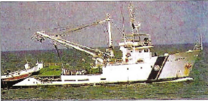
Plate 8: K. L. CERMIN, a 250 GRT training vessel, equipped with a FURUNO scientific echo sounder FQ-70M, used for the acoustic and oceanographic surveys.
