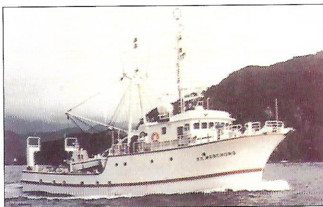
Plate 1: K.K. MANCHONG, 150GRT, research trawler used during the Fisheries Resources Surveys in the EEZ Malaysia, 1997-1999, based at FRI, Sarawak Branch, Bintawa, Kuching. Overall length 27.5 m, draft 2.2 m, trial speed 12.48 knots, crew complement 22 persons.
