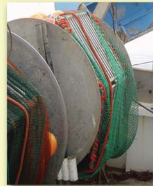
Turtle Excluder Device (TED) from Swedish technology could be hauled in the net drum.
