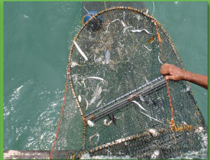
A JTED being hauled onboard after testing.
