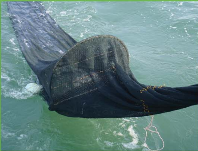
A JTED fixed to a fish trawl ready for testing.
